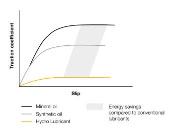
In this scenario, the traction coefficient corresponds to around one tenth of the value that can be achieved with the best available oil-based lubricants, which results in a whole range of positive effects. These range from energy savings and reduced emissions to longer life cycles of different components.
